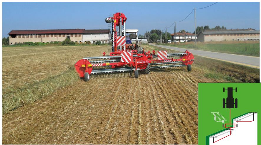
Used in single side-windrow configuration, this rake works well with any quantity of fodder. It is possible to form lateral windrows with one or two passes or to merge multiple windrows to increase the volume of the swath and facilitate the use of the baler.
