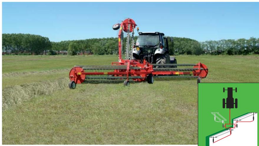
Used in single side-windrow configuration, this rake works well with any quantity of fodder. It is possible to form lateral windrows with one or two passes or to merge multiple windrows to increase the volume of the swath and facilitate the use of the baler.
